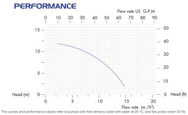
These data may vary according to the construction materials and hydraulic conditions.
