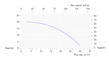
The curves and performance values refer to pumps with free delivery outlet with water at 20 °C, and two poles motor 50 Hz. These data may vary according to the construction materials and hydraulic conditions.
