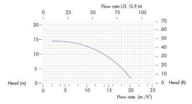
The curves and performance values refer to pumps with free delivery outlet with water at 20  $^{\circ}$ C, and two poles motor 50 Hz. These data may vary according to the construction materials and hydraulic conditions.
