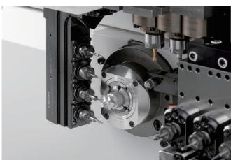
The latest NC unit is installed. This enables simultaneous 5-axis control, and machining of contoured surfaces with highly flexible tool movements. In addition, program processing capability is greatly improved, and cycle times can be shortened.
