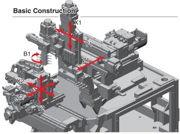
The B-axis machining range for the front spindle has been expanded to 110°. This provides greater flexibility in the machining balance, by reducing the number of tools assigned to back machining for example. In addition, the number of turning tools has been increased from five to six, resolving tool shortages.
