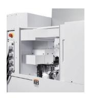
The cutting room door is a flip-up type with a builtin damper, and provides a wide opening for good operating convenience. The larger window also improves visibility when the door is closed.
