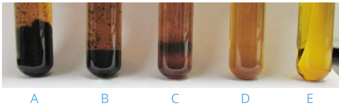
Figure 1 – Deposition Tendency Test
