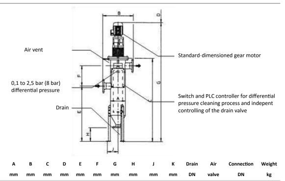
Heco standard filters type AKS are supplied in stainless acid-proof steel EN 1.4404. The filter element is fully welded in stainless acid-proof steel EN 1.4404.
