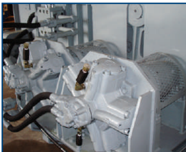
CH clutch mounts between motor and winch
