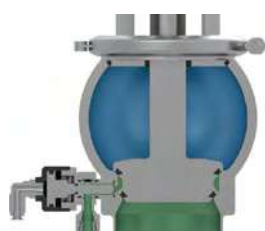
Detection of leakage with only one flushing valve
