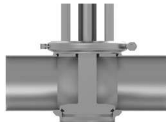
Simple shut-off with only one seal
