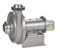
Stainless steel hygienic centrifugal pumps, which are used for pumping liquids up to 300 cP. Depending on the product to be pumped, the pumps can be supplied with a closed impeller, a half open impeller or an open impeller (suitable for pumping liquids with solids).
