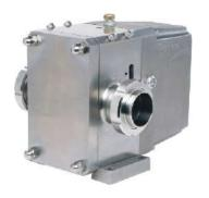
Pomac PLP Lobe pumps are designed to pump high-viscosity liquids (up to 100.000 cP). The pump section and gearbox are made of stainless steel. The pump can easily be cleaned, which reduces its maintenance time. The pump can be mounted with the connections placed vertically (in "self-draining position").
