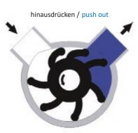
KIESEL Impeller pumps are self-priming pumps. They unite the characteristics of a rotary pump and a positive displacement pump into one.
