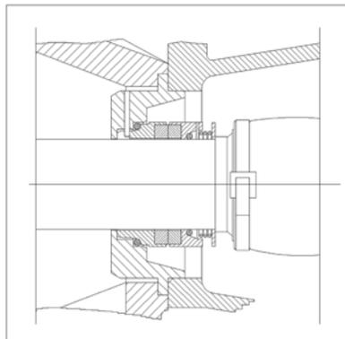
Mechanical seal single-acting, independent of the direction of rotation (open spring element)
