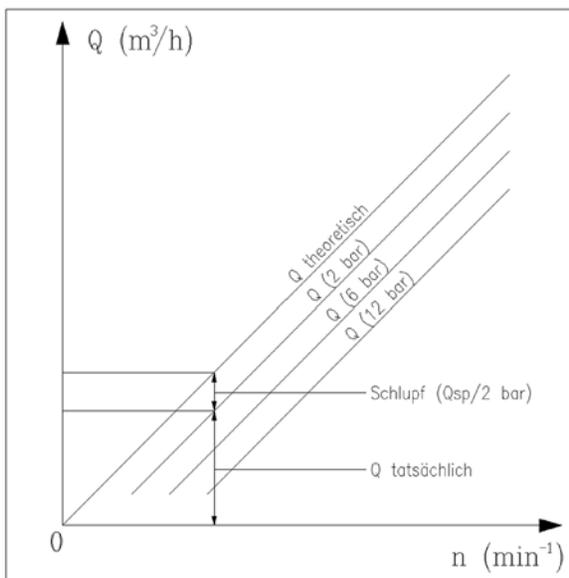
The propulsion characteristics of eccentric screw pumps  $Q$  independent of the number of revolutions.
