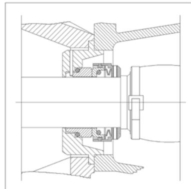
Mechanical seal single-acting, independent of the direction of rotation (open spring element totally sealed)
