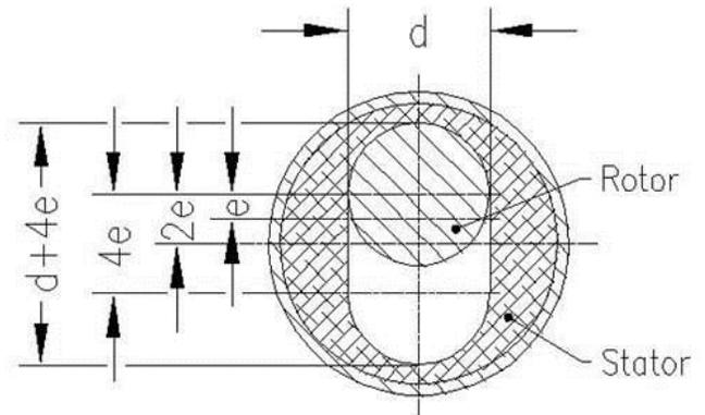
The dimensions at the stator enable the rotor to revolve in it without any play. Consequently the propulsion height— $Q$  does not permit any back-flow. If the propulsion height is greater, the  $Q_{sp}$  increases linearly. Whereupon the dimension tolerances of the stator and the rotor as well as the elasticity of the stator are decisive. The viscosity and temperature of the fluids also have a great impact on the situation.
