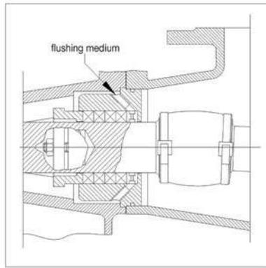
Standard gland packing with soft packing and flush ring for strongly abrasive, crystalline media
