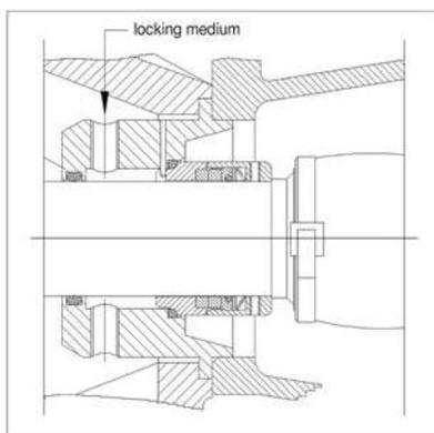
Mechanical seal single-acting, independent of the direction of rotation with quench for clean use
