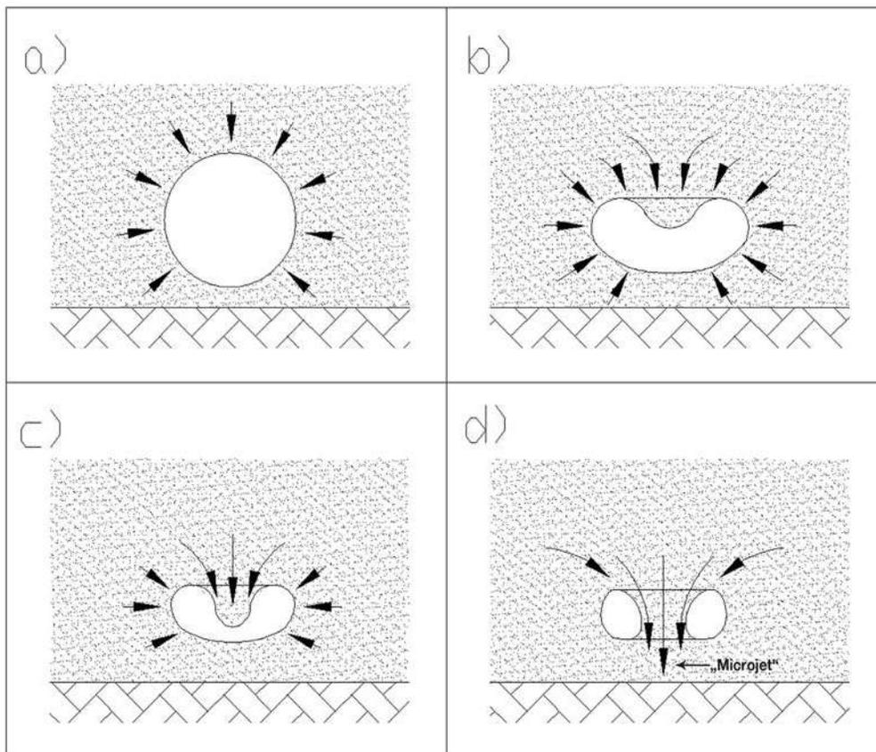
At the beginning of the implosion the generally rounded bubbles (a) become indented (b). With those near to the wall indentation takes place on the averted side. With bubbles in mid-flow indentation takes place on the side with the greater pressure.
