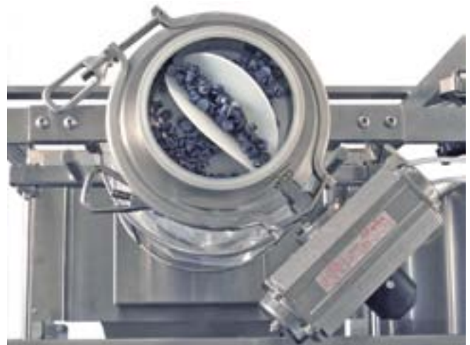
Dettaglio ROTARY VALVE TABLET con tappi in silicone Detail of ROTARY VALVE TABLET with silicon caps
