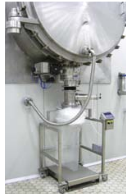
Sistema dosaggio liner continuo, scarico e dosaggio paddle dryer Continuous liner dosing system, discharge and dosing from a paddle dryer
