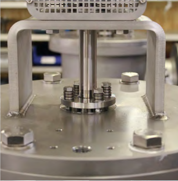
Spring loaded sealing box for tight sealing
