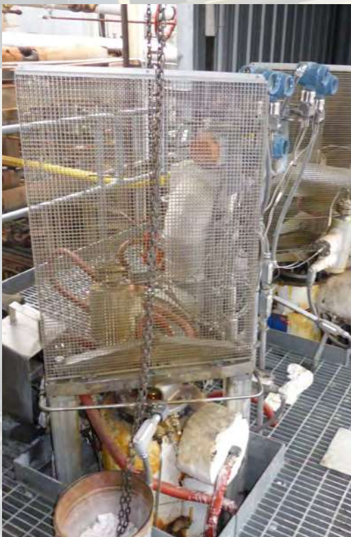
Filtration of natural resin at 275°C, 100 µm defined pore filtration.
