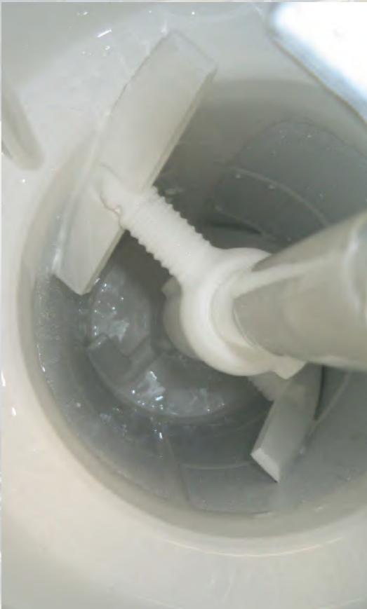
Solid spring loaded rotating scraper system.
